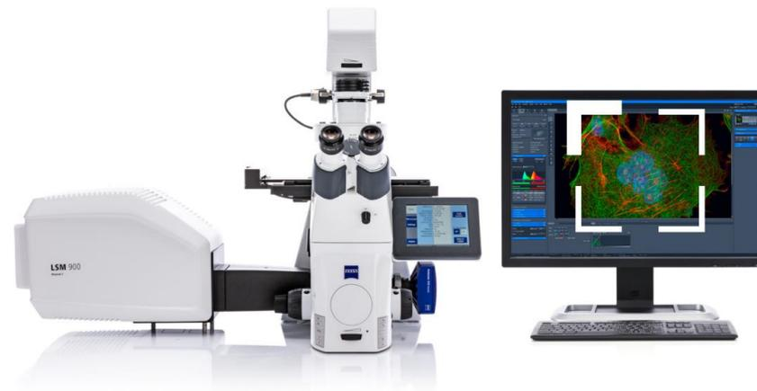
**ZEISS LSM 900 with Airyscan 2**
